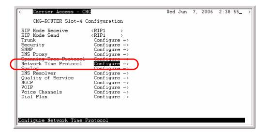
2. To enable Network Time Protocol, scroll **<Disabled>** to **<Enabled>**, with the **[SPACEBAR]**, select **[ENTER]**.
